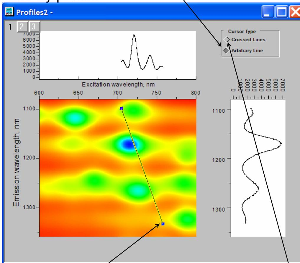
Grab an end of the profile line and move to the desired location on the matrix. The profiles are updated.
