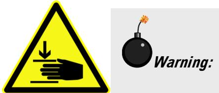
Danger to fingers! This symbol warns the user that the equipment is heavy, and can crush or injure the hand if precautions are not taken.
