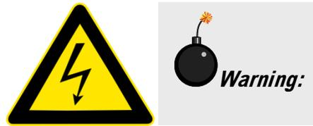
Risk of electric shock! This symbol warns the user that un-insulated voltage within the unit may have sufficient magnitude to cause electric shock.
