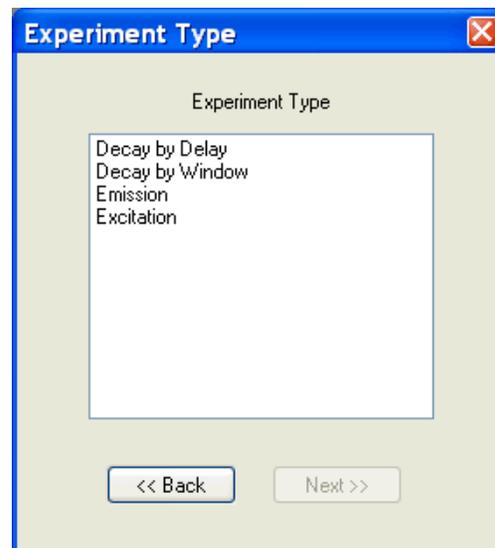
**Excitation** These are similar to the standard excitation, and emission scans. Among the changes are that the **Integration Time** field is removed, and instead are data-entry fields for **Sample window**, **Delay after flash**, **Time per flash**, and **Flash count**. These four fields are described above, in the **Theory of Operation** section, and shown below (extracted from the **Experiment Setup** window).
