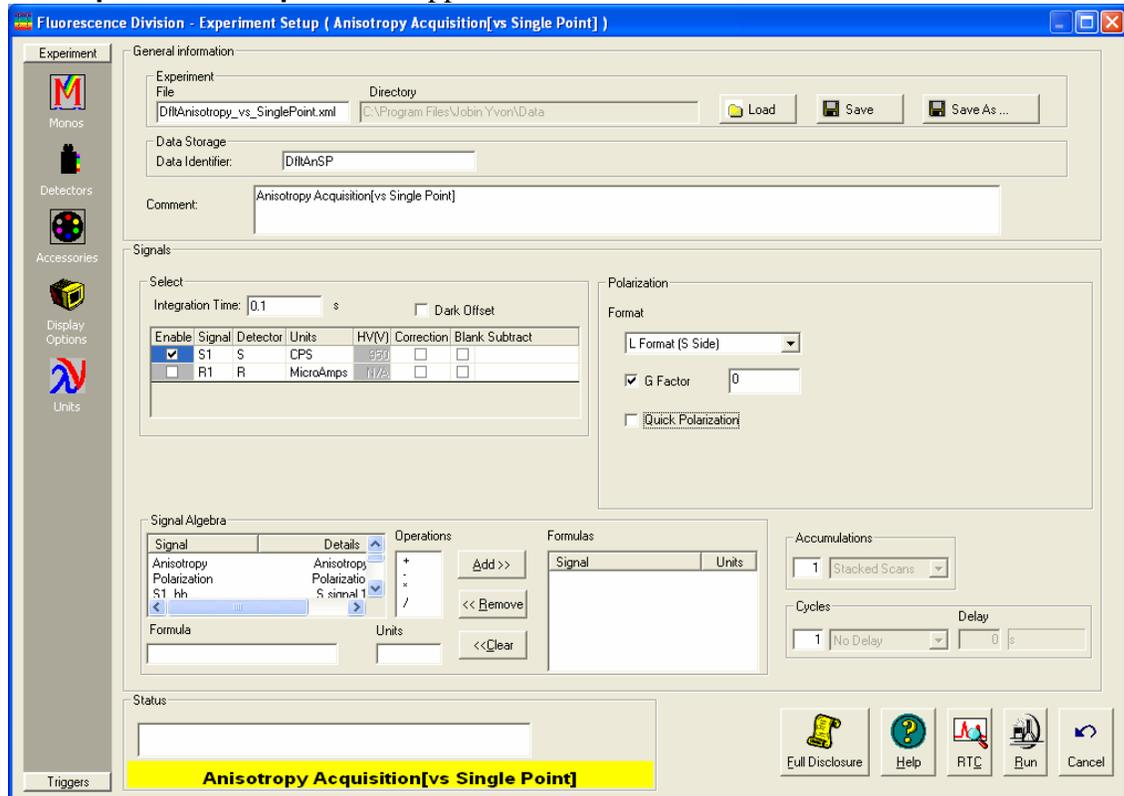
Use the appropriate **Signal** in the **Signal Algebra** area. Add >> it to the **Formulas** table. To cause the instrument to measure any *G* factor(s), disable the **G factor** checkbox during the scan. To specify *G* factor(s) beforehand, enter the *G* factor in the field.
