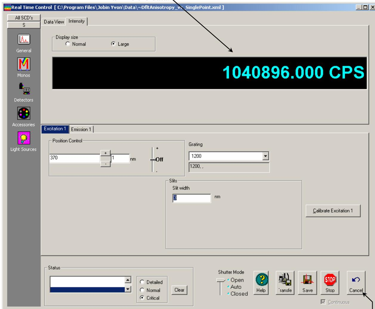
The value should be  $\sim 1 \times 10^6$  cps. If the signal is  $> 2 \times 10^6$  cps, then dilute your scatterer. If the signal is  $< 2.5 \times 10^5$  cps, add more scatterer to increase its concentration. You may also adjust slits, but keep them between 3–5 nm for best results.
