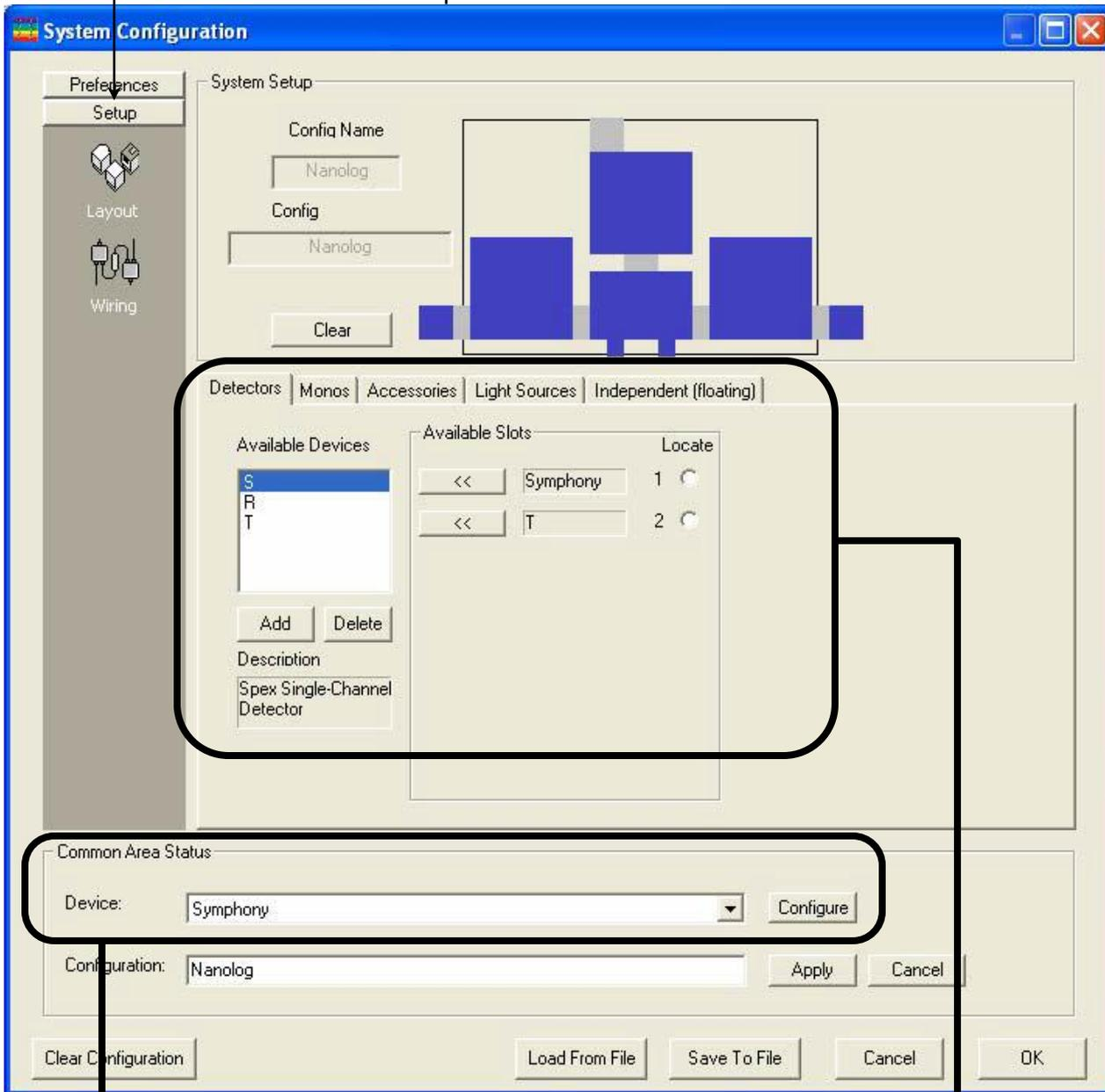
e Choose the Detectors tab, S, from the Available Devices area, and confirm that the Symphony<sup>®</sup> or other special detector/controller combination is correct in the Available Slots area.
