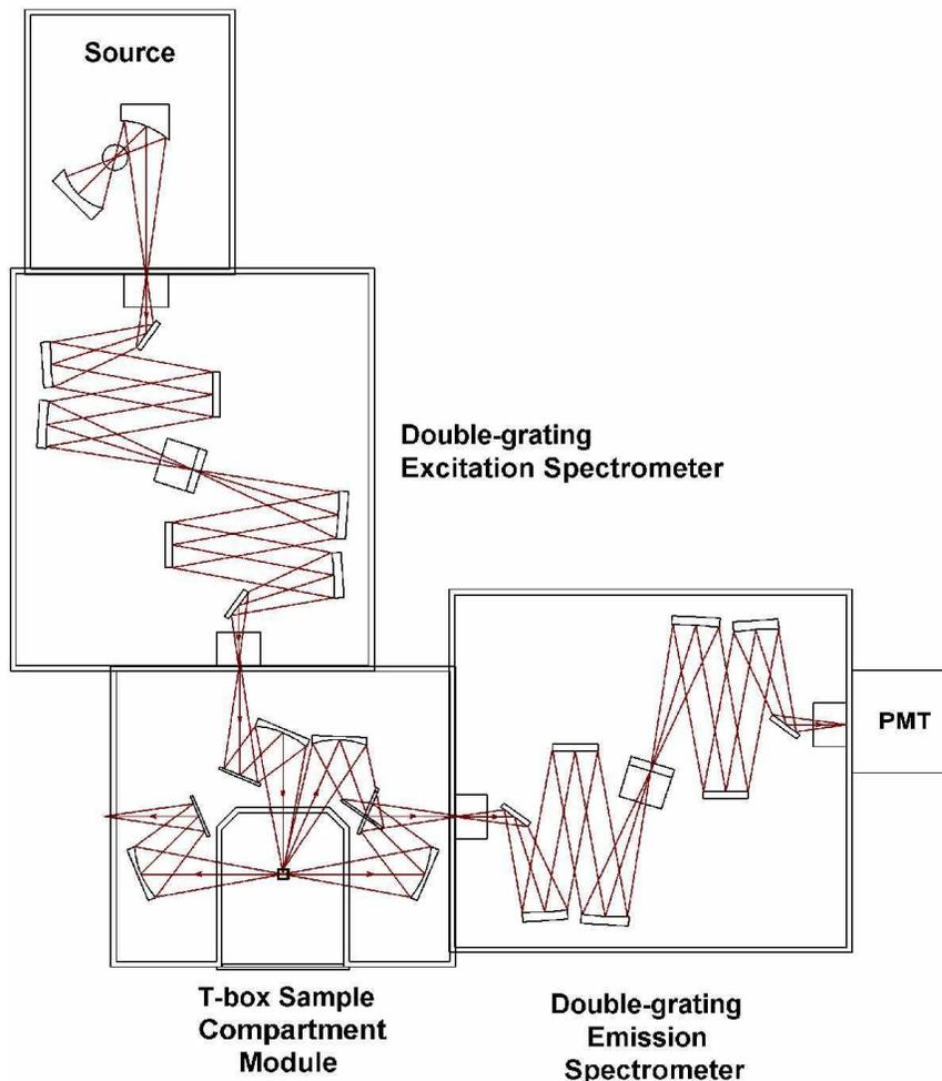
Incorporating double-grating monochromators in both the excitation and emission positions places this model in a category by itself. Enhanced features, modular structure, and few external controls are just a few of the reasons to consider a Fluorolog<sup>®</sup>-3 model FL3-22:
