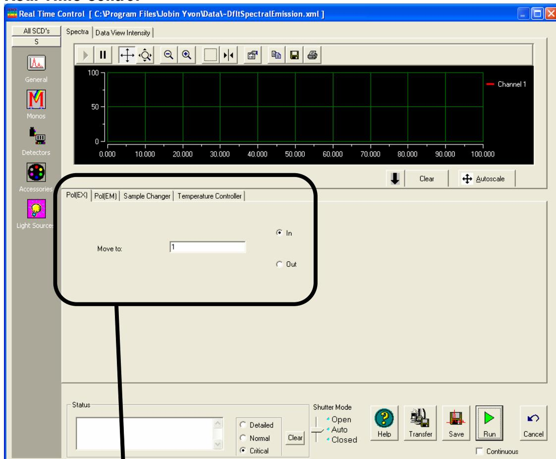
**Real Time Control** manipulates the polarizers and other instrument settings, to observe and optimize the spectrofluorometer in real time. Under the **Accessories** icon in the **Experiment Setup** window, each polarizer may be set independently into or out of the optical path under its own index-card tab. A custom angle may be set from 0–180°, in the field provided.
