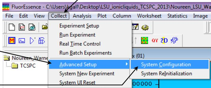
If the system has not been initialized, choose the instrument, and let the system initialize. Then redo steps 1–3. The **System Configuration** window appears:
