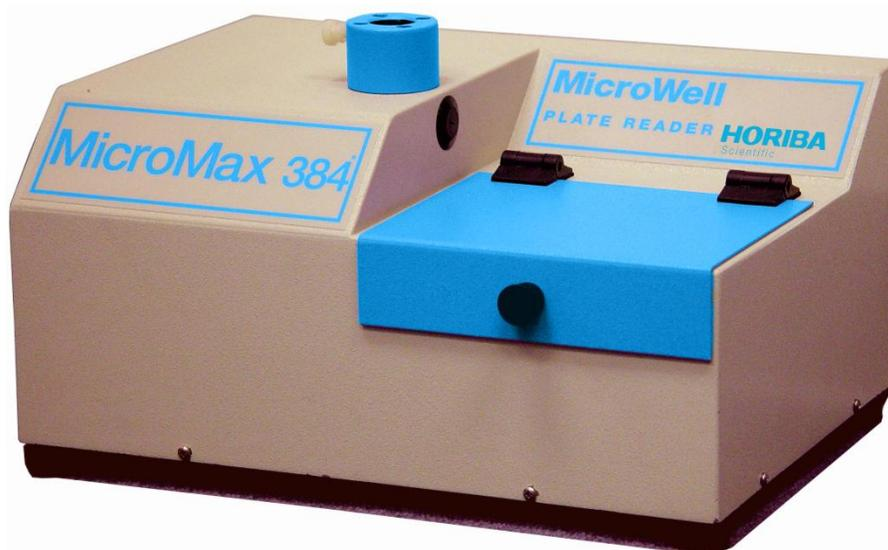
The MicroMax 384 Microwell Titer-Plate Reader allows multiple samples to be scanned in one experiment. The MicroMax 384 is controlled through FluorEssence™ software via a serial port to the host computer. The titer plate moves beneath a stationary optical beam, and fluorescence measurements are collected with top-reading geometry. Thus, any titer plates—even disposable ones—may be used. Plates with 96 and 384 wells may be inserted into the MicroMax 384, with a scan speed < 1 min for all plates.
