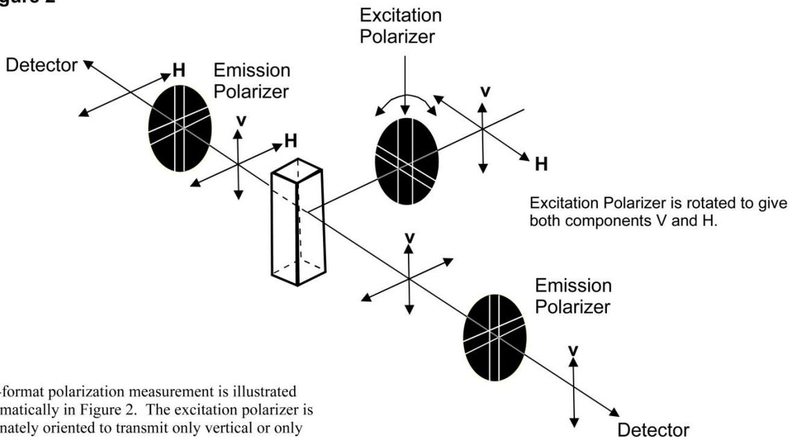
A T-format polarization measurement is illustrated schematically in Figure 2. The excitation polarizer is alternately oriented to transmit only vertical or only horizontal components of the excitation radiation to the sample. Dual emission paths, each with a polarizer, permit simultaneous measurement of the vertical and horizontal components of the emitted luminescence.
