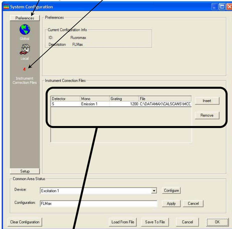
The Instrument Correction Files area should display a correction file for the Detector (S or R). If not, click the Insert button, and browse for the desired correction file.
