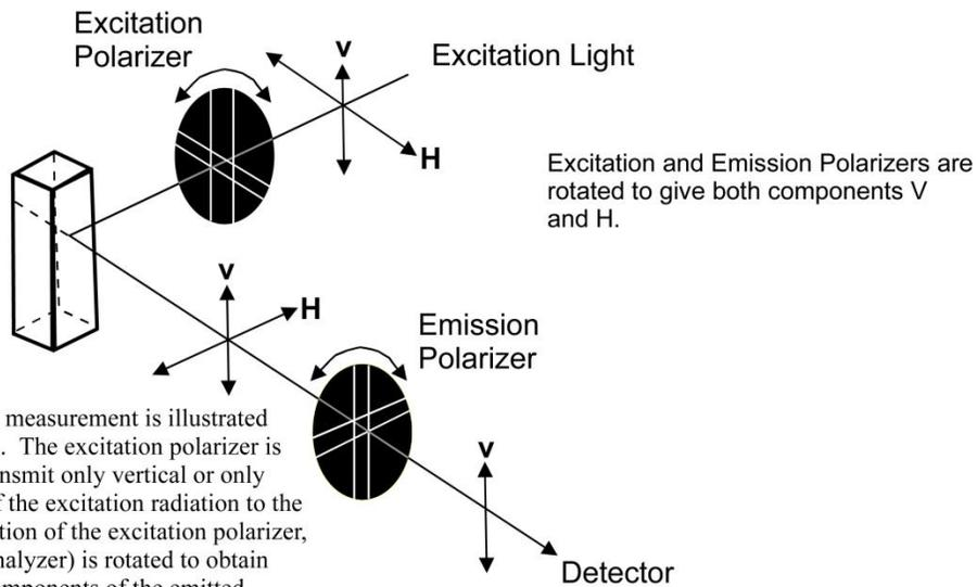
An L-format polarization measurement is illustrated schematically in Figure 1. The excitation polarizer is alternately oriented to transmit only vertical or only horizontal components of the excitation radiation to the sample. For each orientation of the excitation polarizer, the emission polarizer (analyzer) is rotated to obtain vertical and horizontal components of the emitted luminescence.
