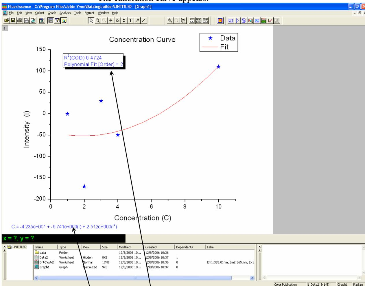
Stars indicate the standards. The unknowns are not plotted, but their calculated concentrations are filled in on the dataset. The fit equation and correlation are displayed on the plot.
