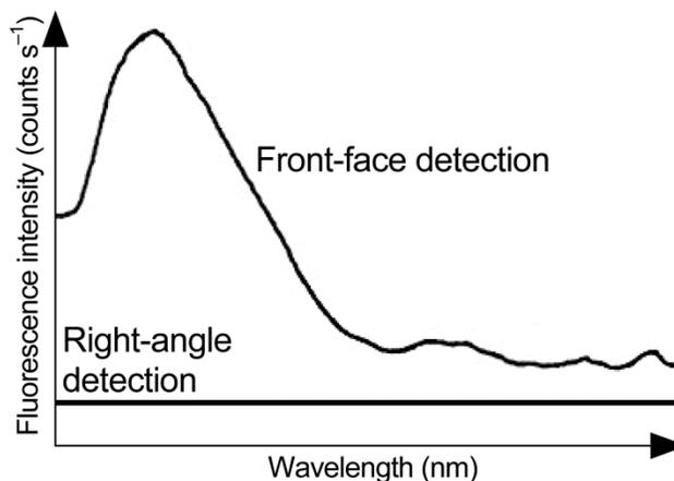
Comparison of fluorescence emission signal from sickle-cell hemoglobin using right-angle versus front-face detection. The  $\beta$ -37 tryptophan is primarily responsible for this fluorescence.
