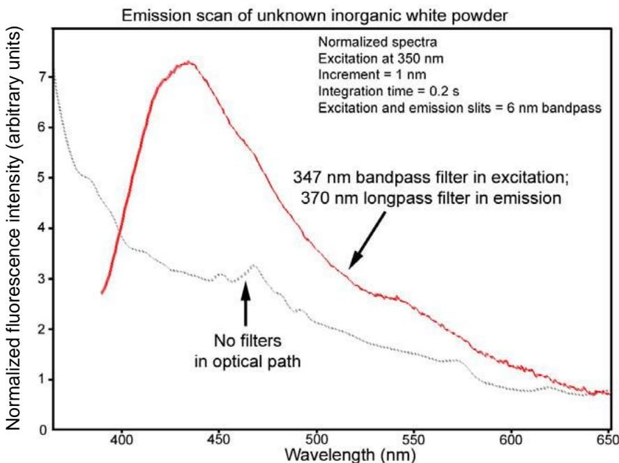
not stray excitation, into the detector. Notice how the shape of the spectrum changes drastically when filters are added.
