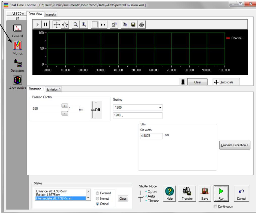
5 In the Emission 1 tab, enter 397.00 in the Position Control, then slide the Shutter Mode switch to Open.
