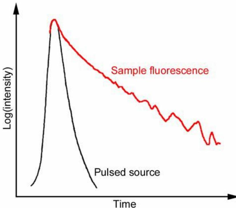
Schematic of time-domain lifetime measurements.
