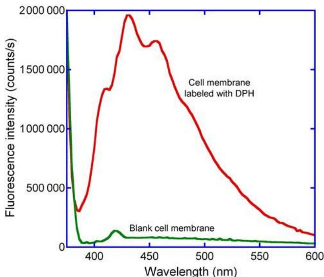
The cell membrane tagged with 1  $\mu\text{M}$  DPH is detected easily in this graph.
