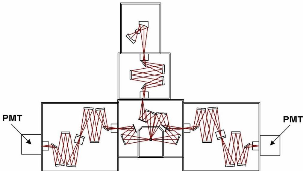
**Optical layout of the Fluorolog<sup>®</sup>-3 Model FL3-122.**
