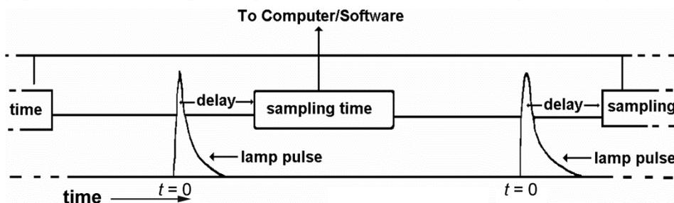
for a pre-determined length of time (the Sample Window). Any signal arriving before or after the gating is ignored. To increase or decrease the signal, you can adjust the time per flash and the sample window.
