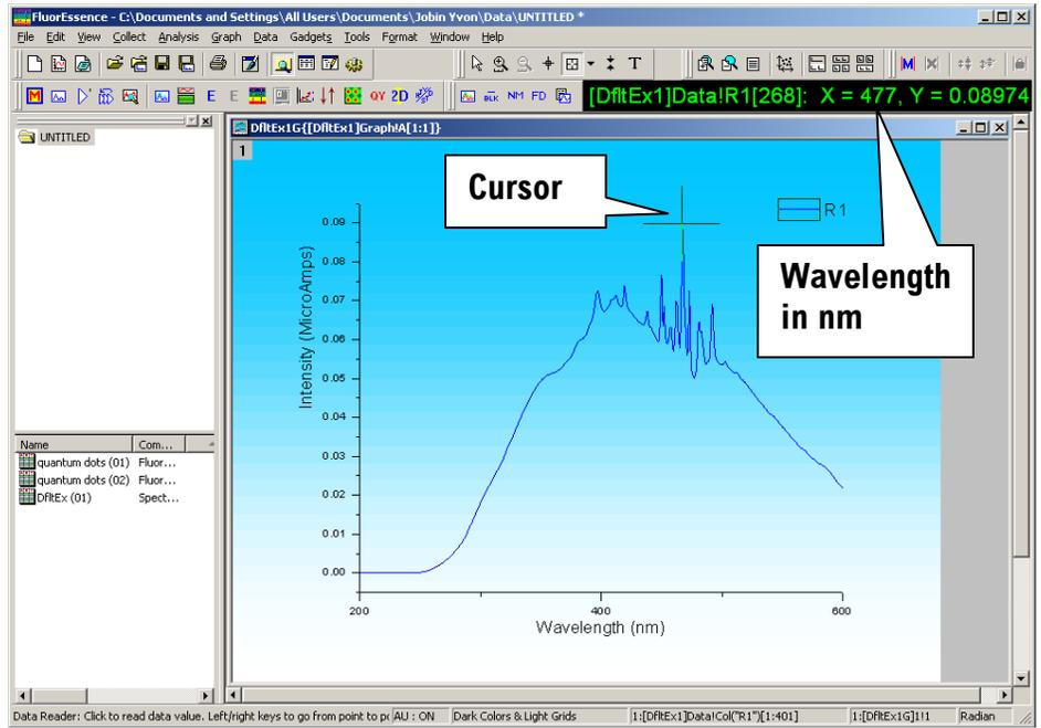
This example shows the peak actually at 477 nm, which is 10 nm too high. Therefore we must recalibrate the monochromator.
