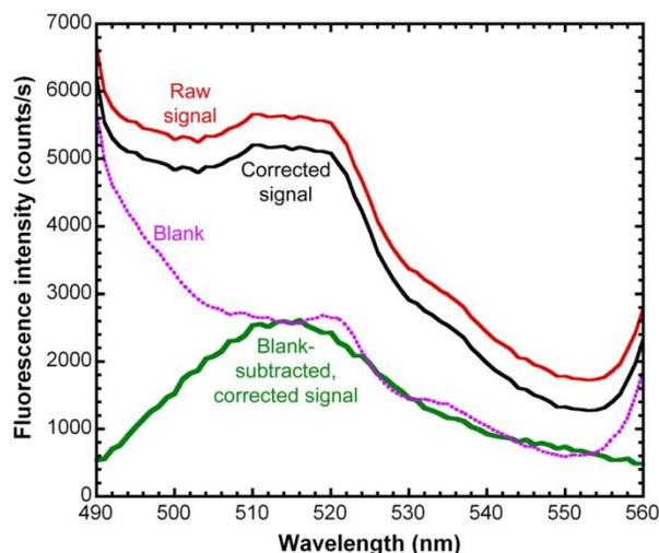
Single-scan emission (no smoothing) from 50 fM fluorescein in 0.01 M NaOH. Note the H-O-H Raman bending mode at 521 nm in both blank and sample.
