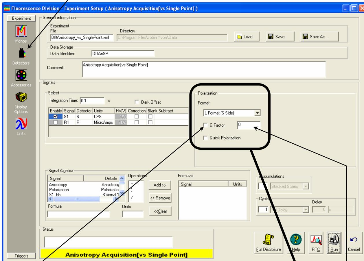
This shows the parameters related to detectors, including the *G* factor, in the Polarization area.
