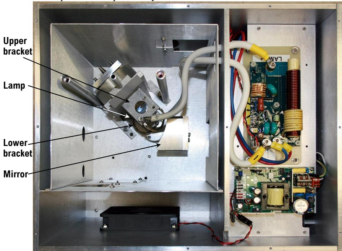
Top view of the lamp housing with cover removed.
