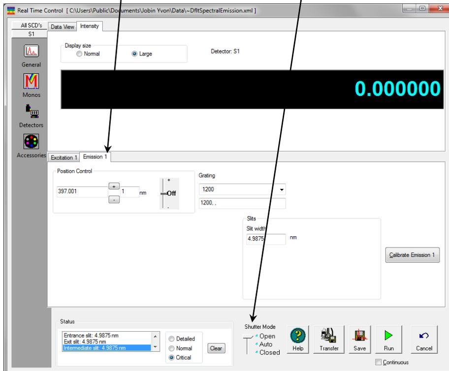
6 Click the Detectors icon, and slow the Integration Time to about 0.3–0.5 s. This makes it easier to adjust the lamp without missing the maximum signal.
