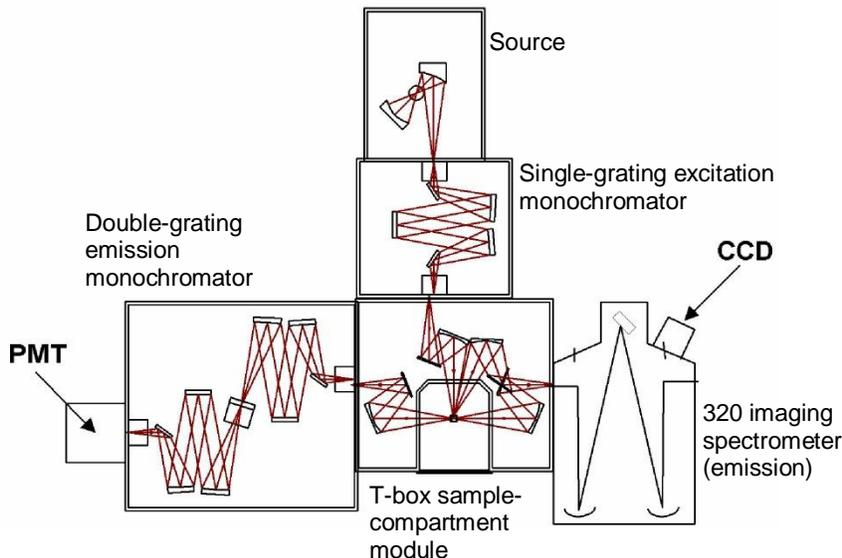
**Custom optical layout. By switching the iHR320 and double-grating monochromator, both right-angle and front-face collection are possible.**
