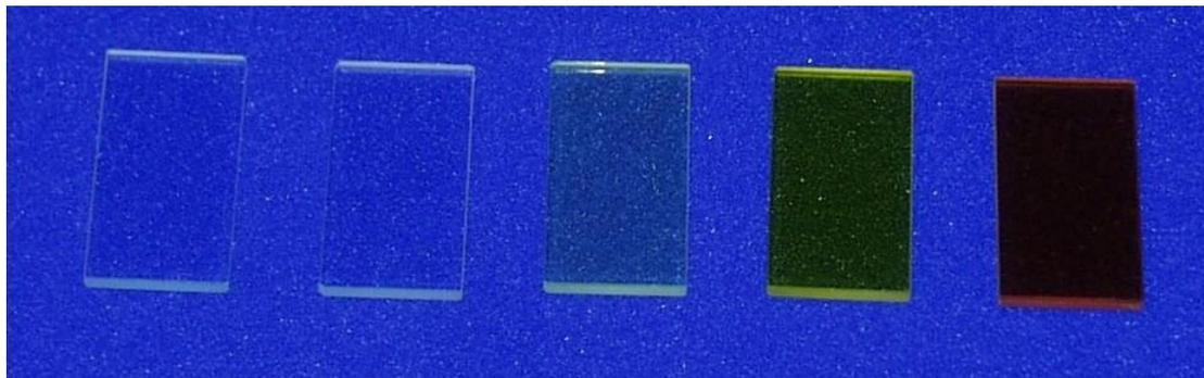
The J1938 Cut-On Filter Set consists of 5 filters with dimensions of 1"  $\times$  2" (2.5 cm  $\times$  5 cm). To properly position the filter, the FL-1010 Filter Holder is required.
