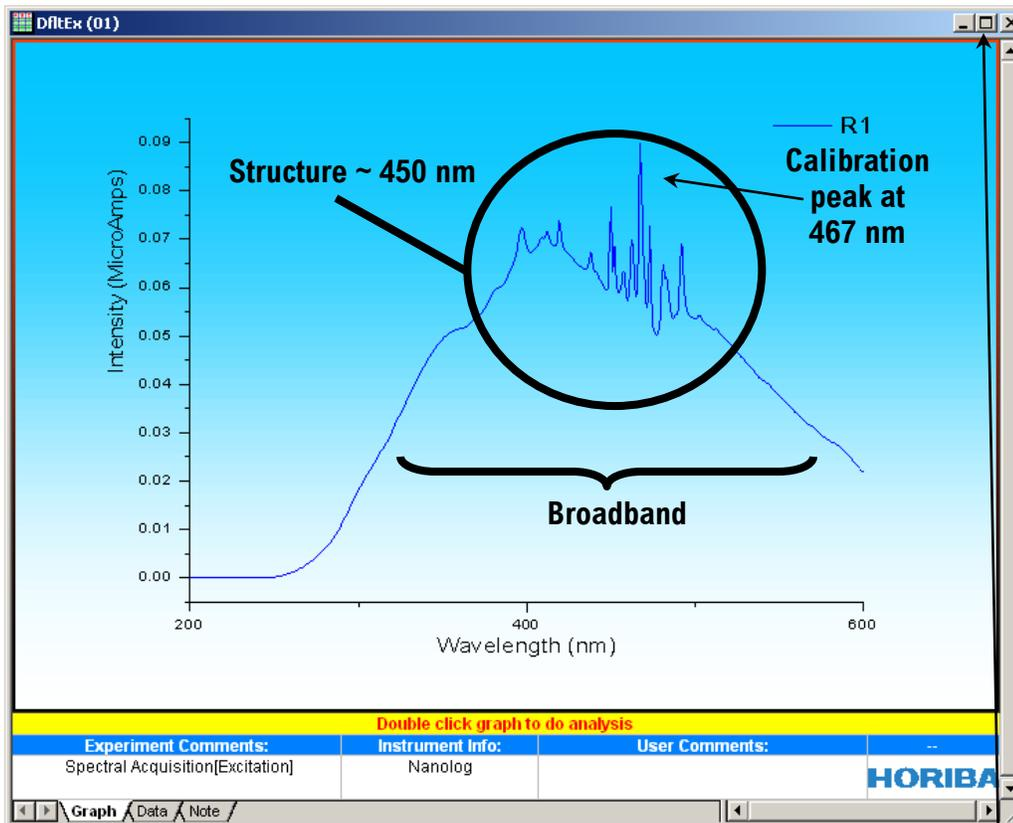
This is an uncalibrated FluoroMax lamp scan. The main peak ought to be at 467 nm, but here appears near 480 nm.
