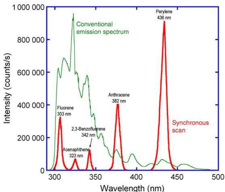
The solid line in the figure above is the emission spectrum acquired on a Fluorolog<sup>®</sup> system (single-grating monochromators) with constant wavelength excitation. As shown by the broken line, when the sample is scanned synchronously, five individual components are resolved into unique, sharp peaks indicative of the individual compounds.
