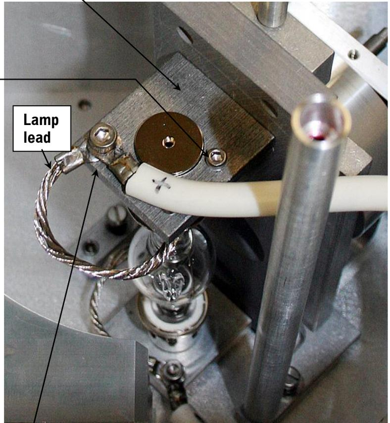
8 Secure the lower lamp lead and lower power cable to the lower bracket, using a 5/32" cap screw.
