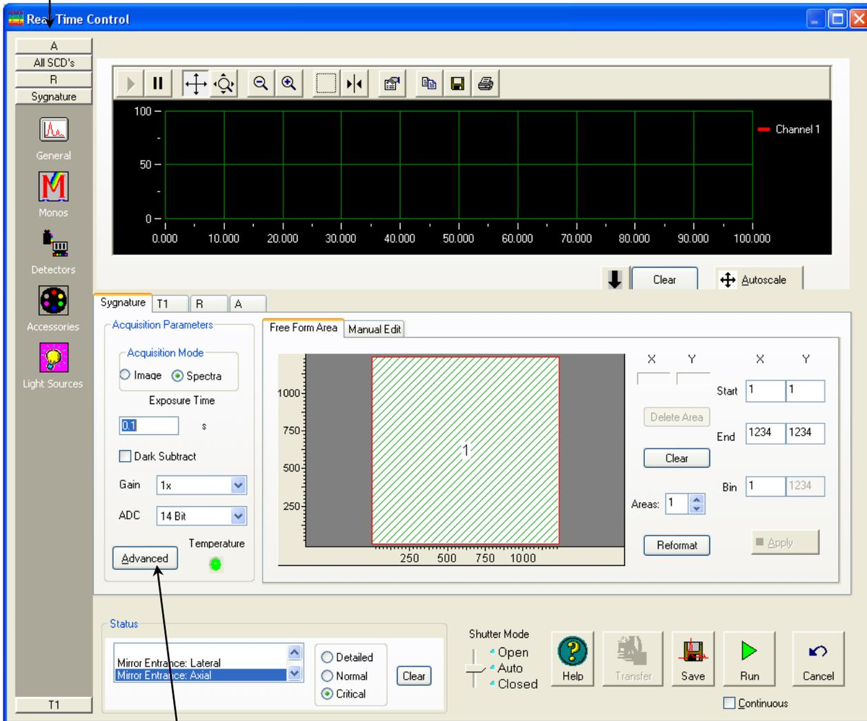
In the Acquisition Parameters area, click the Advanced button to open the **Multichannel Detector Advanced Parameters** window.
