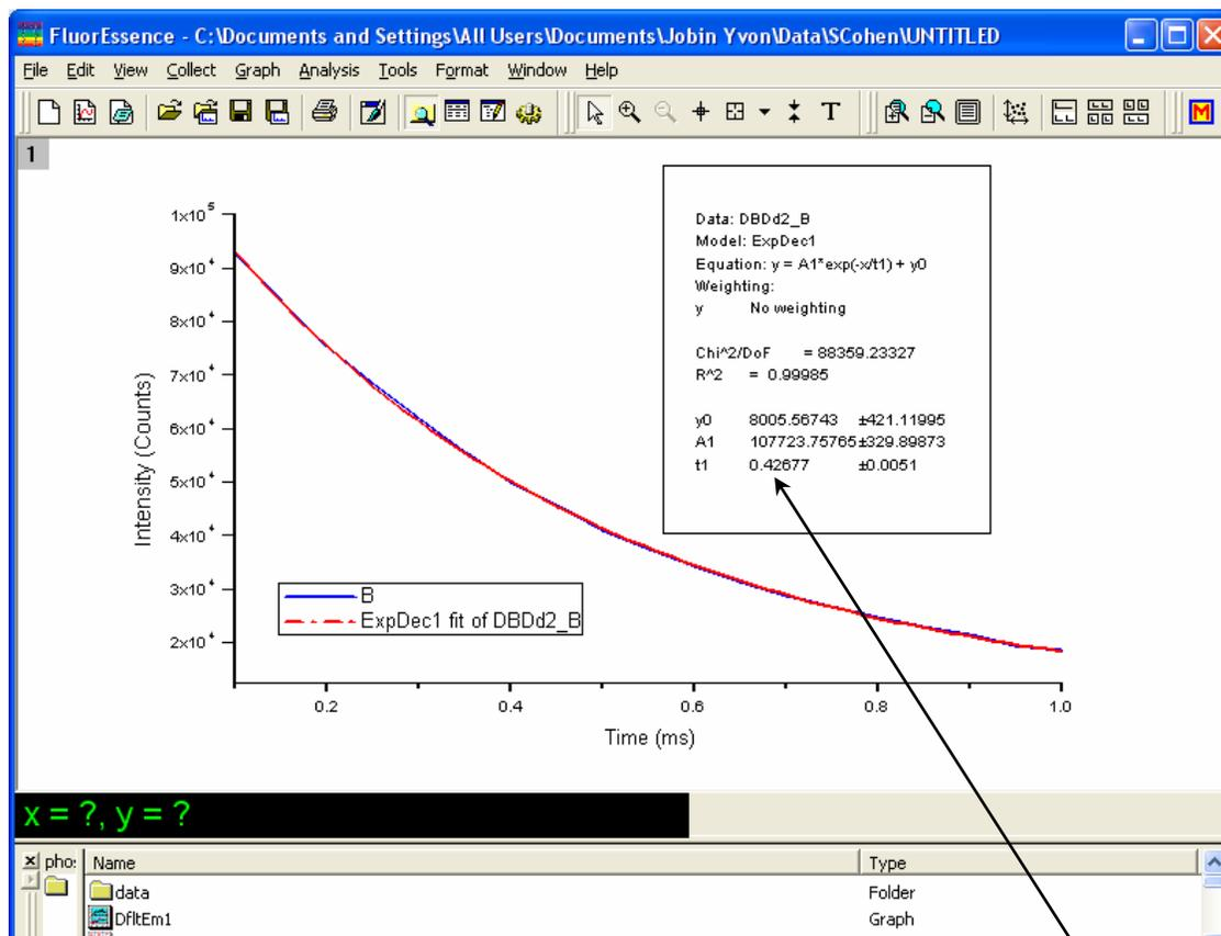
With the **Phos** experiment type in the **Fluorescence Experiment Menu**, create a phosphorescence-decay curve, as in the screenshot from FluorEssence™ shown above. This is an example using data from  $\text{TbCl}_3(aq)$ , fitted to a single-exponential curve-fit in Origin®. All parameters are automatically displayed, including the fitted lifetime of 427  $\mu\text{s}$ .
