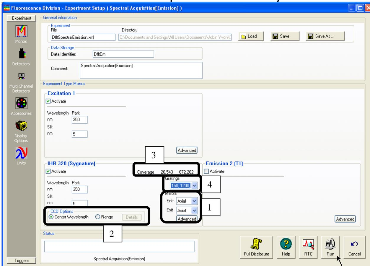
This is an example using an emission scan-type. Under the Monos icon, functions specific to the iHR are available, such as:
