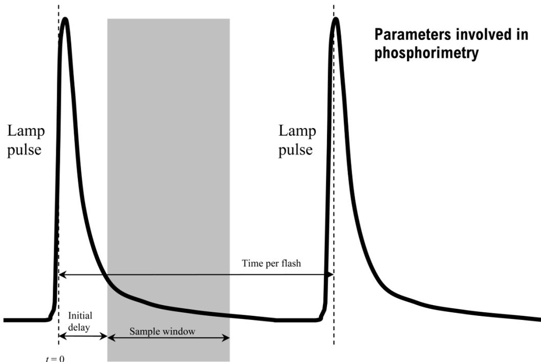
This sequence of excitation, delay, and sampling, is repeated for each lamp flash. The signal is accumulated for a predetermined number of excitation pulses, then FluorEssence™ collects the total signal. After collection, FluorEssence™ displays the intensity of the luminescence as a function of time or wavelength. The x-axis is based on one of the four scan options:
