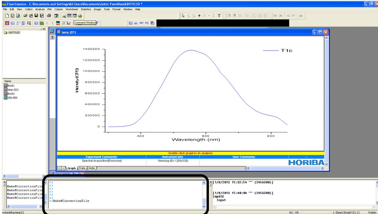
**c** Type MakeMCorrectionFile, then the Enter key. The **Open** window appears.
