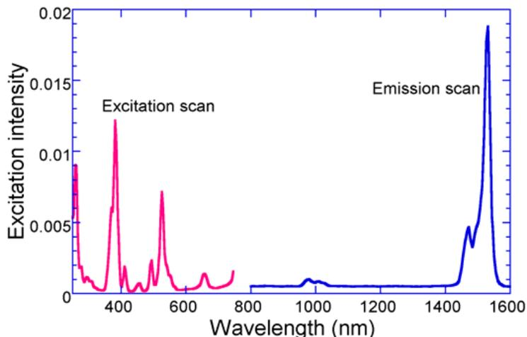
Visible and near-IR spectra of erbium-doped laser-glass acquired on a Fluorolog<sup>®</sup>-3.
