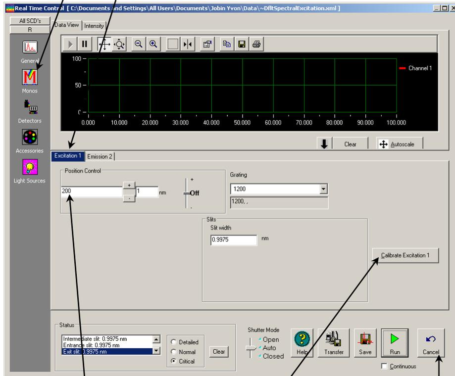
j Enter the current, observed position of the peak in the **Position Control** (here, 477 nm).
