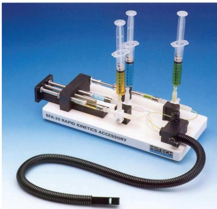
The stopped-flow accessory permits observation of the reaction rate of two reactants forced through a mixing chamber, and into an observation cell. The reactant solutions are contained in drive syringes whose pistons simultaneously are driven. After leaving the observation cell, the reactants advance a stop syringe, triggering data-acquisition by the spectrofluorometer.
