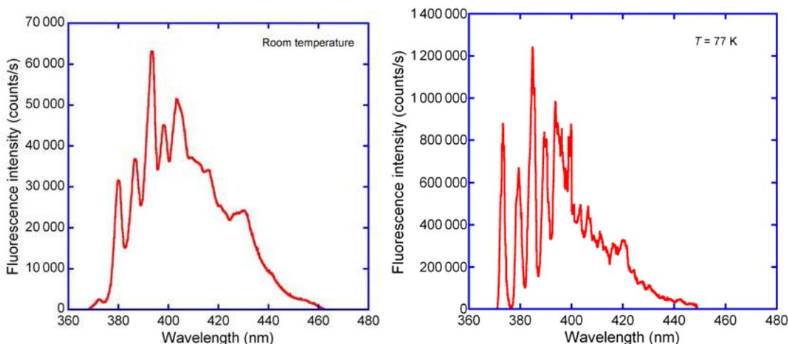
A sample of pyrene at room temperature (left) and at liquid-nitrogen temperature (right). Note the sharper peaks at lower temperature.
