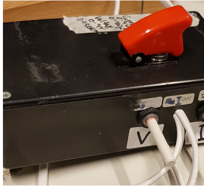
(b) Main controls for daily use, current and voltage dial, enable button
